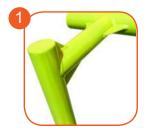
Solid construction made of black steel S235JR, cleaned in the sandblasting process. Protected against corrosion by galvanizing and powder coating with polyester paint QUALICOAT attested.
